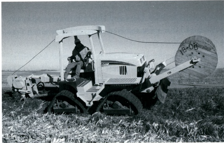
The innovative quad track design of the Vermeer RTX1250 tractor increases side-hill stability and floatation in soft or sandy soils.
