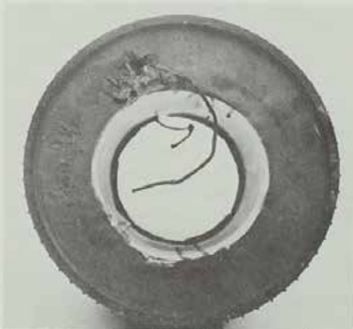
An end view of one of the ABC's memory drums. (courtesy the Department of Special Collections, ISU library)
