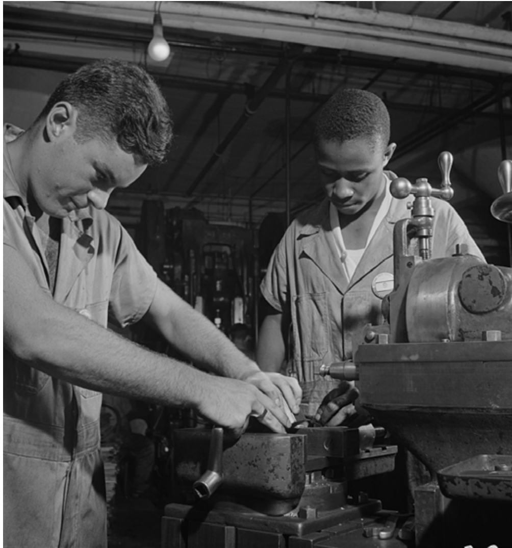
Henle, Fritz, "National Youth Administration work center (NYA), Brooklyn, New York. Two men, white and Negro, who are receiving training in machine shop practice, shown setting up shaper work to cut forty-five degree angles at base for surface gauge," ca. August 1942. Courtesy of Library of Congress
