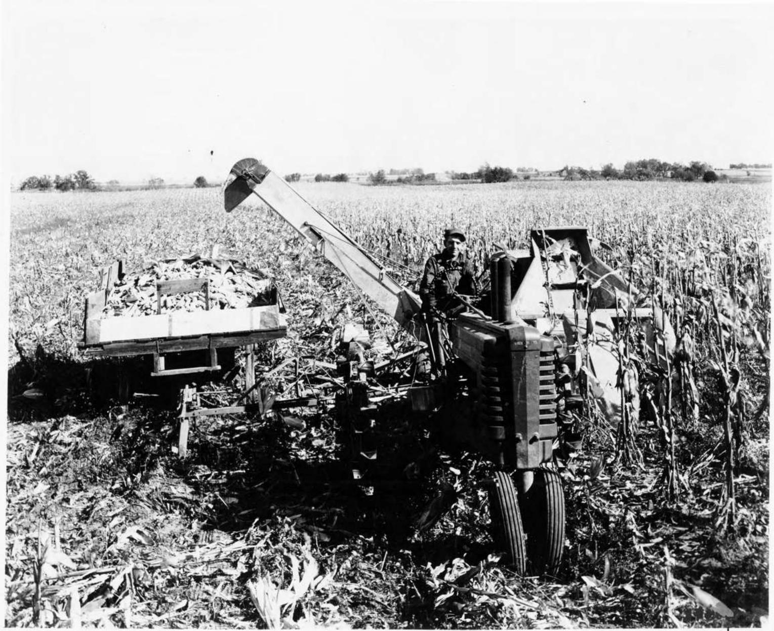
A farmer drives a John Deere tractor with a corn picker and wagon attached. This corn picker harvests the ear from the plant but does not shell the kernels from the cob. That is another step in the farmer's production before selling the corn. *Courtesy of the State Historical Society of Iowa, ca. 1945*
